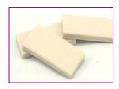
White streak plates are typically used to test dark colored minerals.
